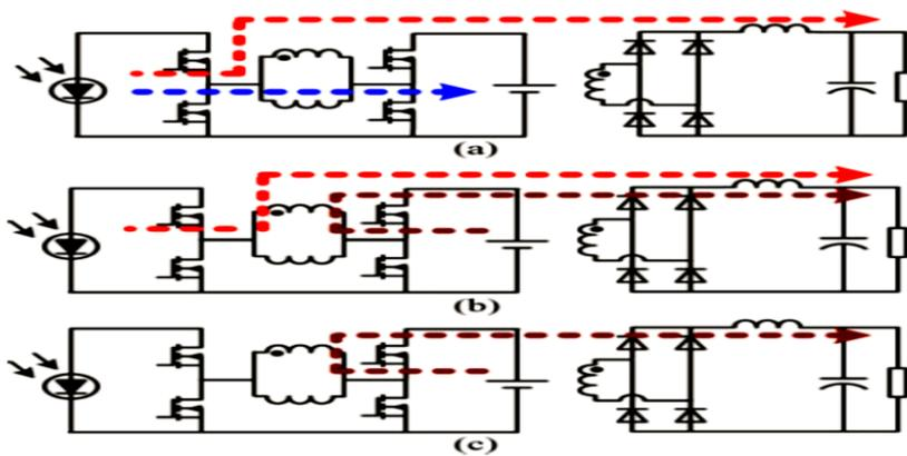
Figure 3. Power flow directions of each operation mode, (a) DO mode. (b) DI mode. (c) SISO mode.
