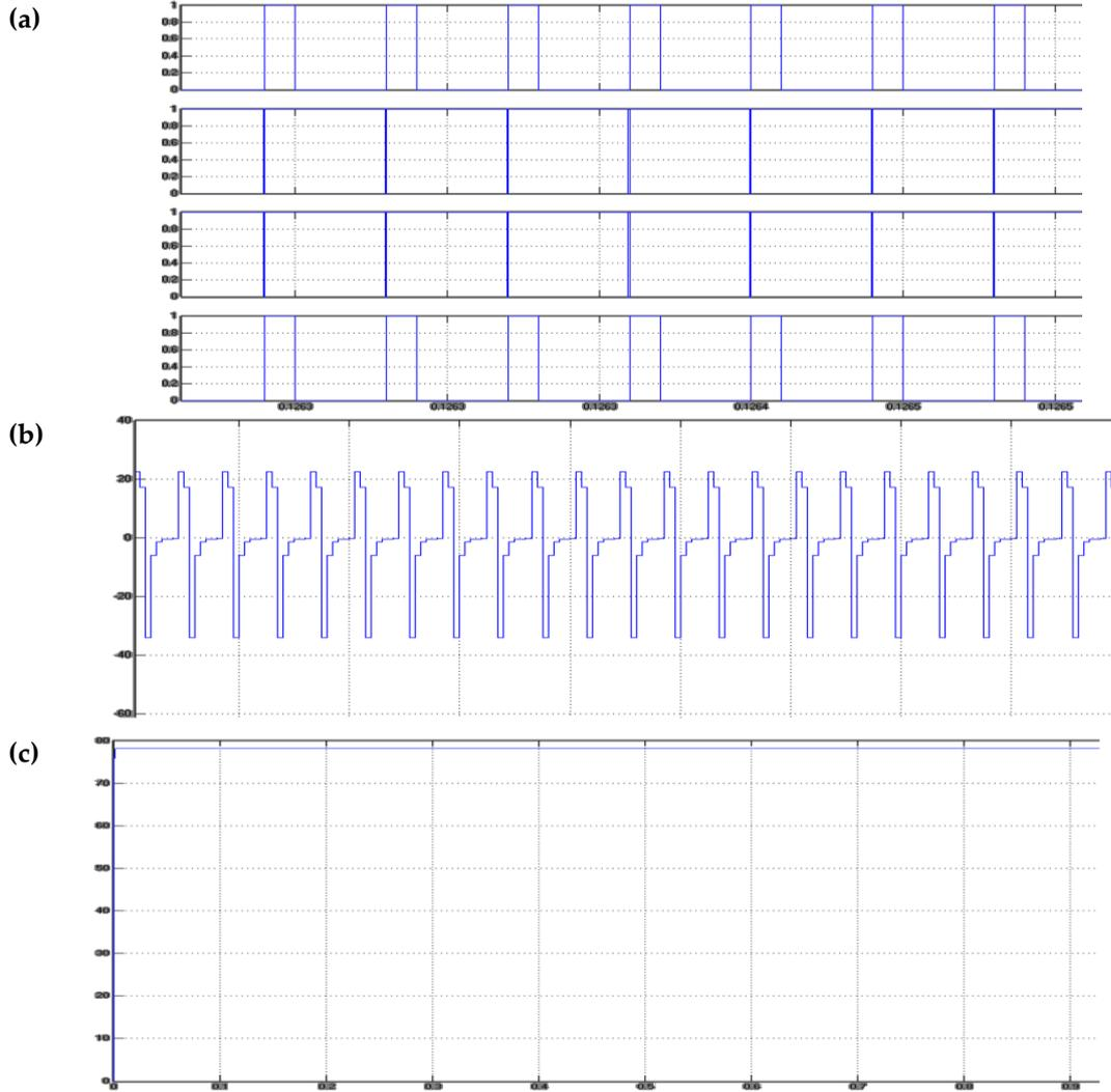
Figure 5. Simulation result for proposed advanced converter, (a) Switching Pulse, (b) Transformer voltage, and (c) Output voltage
