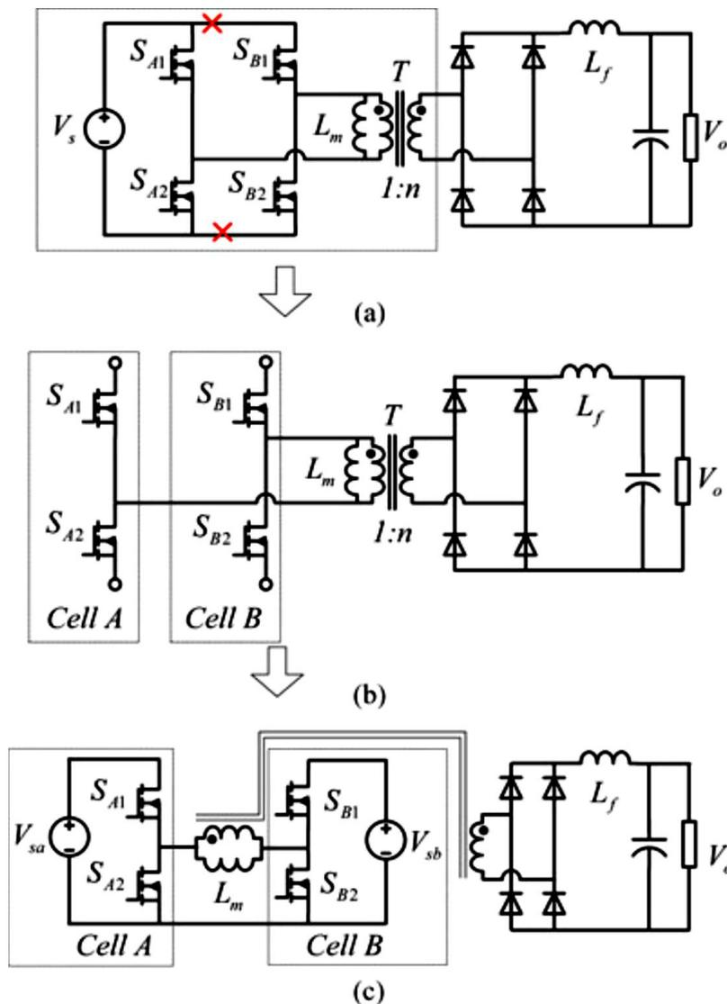
**Figure 1.** Proposed full bridge 3 port converter. (a) Full bridge converter. (b) 2 switching cells. (c) Full bridge 3 port converter
